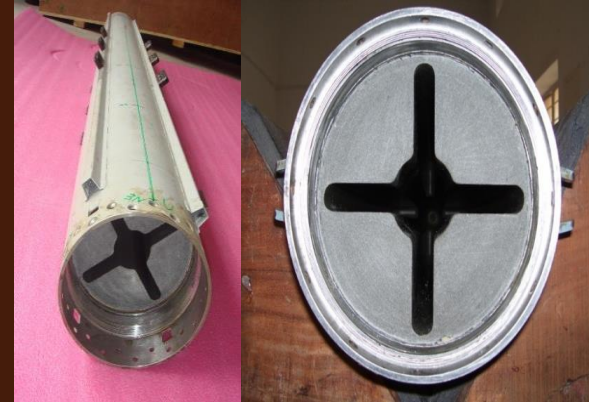
Astra Motor cast with Smoke-less Propellant
