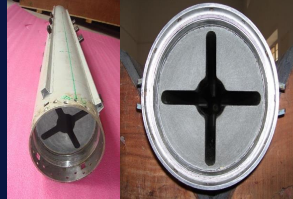
Astra Motor cast with Smoke-less Propellant
